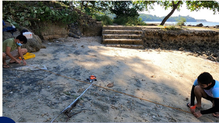
Mark survey area using a 4 m rope. 2
